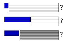
How to divide the memory between sub-TMTO's ? Grid search or metaheuristic search for the average time In this case: speedup of  $16.45~\mbox{w.r.t.}$  single TMTO
