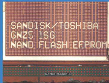
Toshiba 56nm 16Gb MLC NAND Flash Part Die Markings
