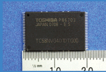
Toshiba 56nm 16Gb MLC NAND Flash Part Package Marking TC58NVG4D1DTG00
